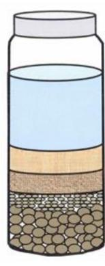
Clay layer – water clears Silt layer – 2 hours Sand layers – 1 minute
